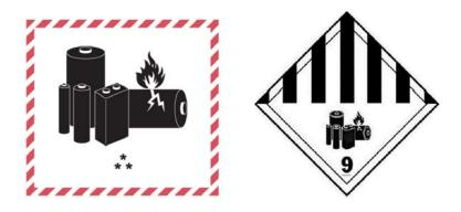
There is no hazards in accordance with the UN recommendations tests (Manual of Tests and Criteria, Part III, sub-section 38.3, 1.2m Drop)
